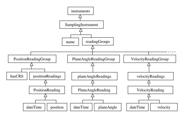
Fig. 5. Proposal for representing instruments within DIGGS (after Bray, 2007)
