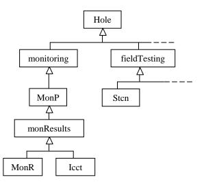
Fig. 2. AGSML representation of monitoring data (after AGS, 2005)
