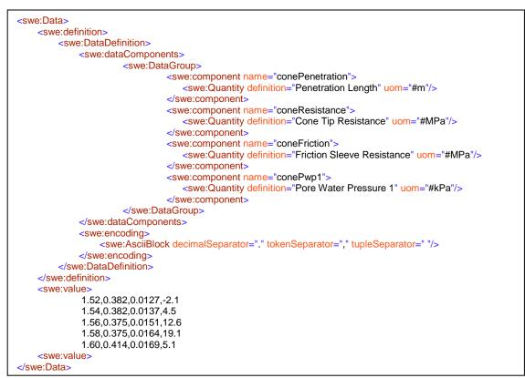
Fig. 6. An example of SensorML for CPT data
